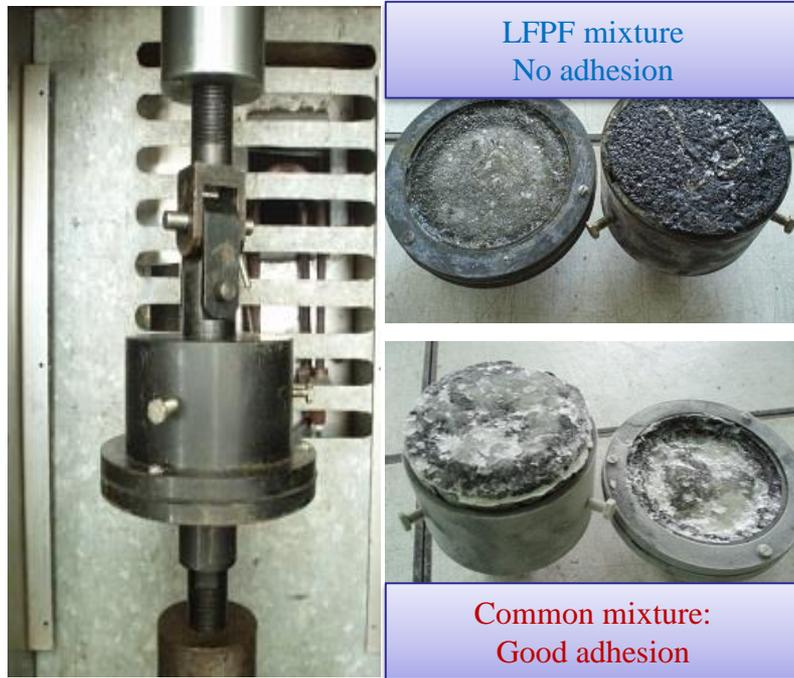
The device evaluating the adhesion property between ice and asphalt mixture
